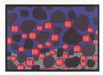
The HYDROCAP then forms non-soluble crystalline structures that prevent the penetration of liquid.
